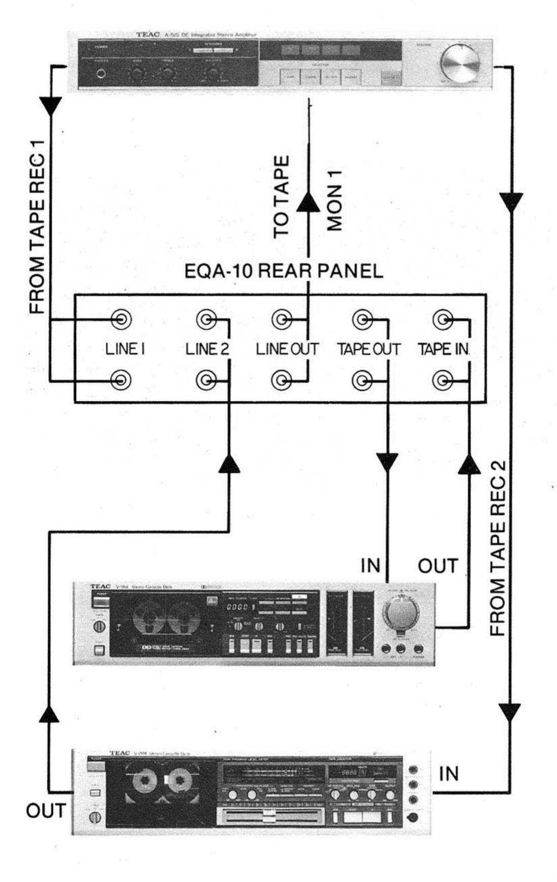
The suggested hookup shows a method of monitoring either of two cassette decks through the EQA-10 so that their recorded programs may be equalized as they are played. The main deck may be used to make equalized copies from the second deck, and if your amplifier or receiver has facilities for dubbing tape 1 to tape 2, you can also switch EQA-10's SOURCE/TAPE SWITCH to tape (down position - LED on) and make an equalized copy from the main deck to the second deck.
