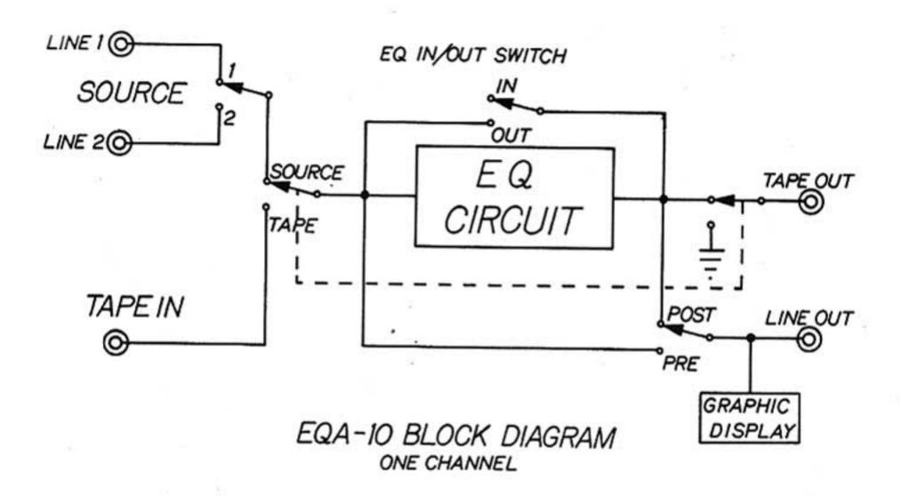
A block diagram is a roadmap of signal flow. Signals usually flow from left to right. As you can see, the EQA-10 is very simple.
