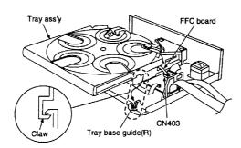
1. Fit the claws on the right side of the tray ass'y underneath the claws on the tray base guide(R).
