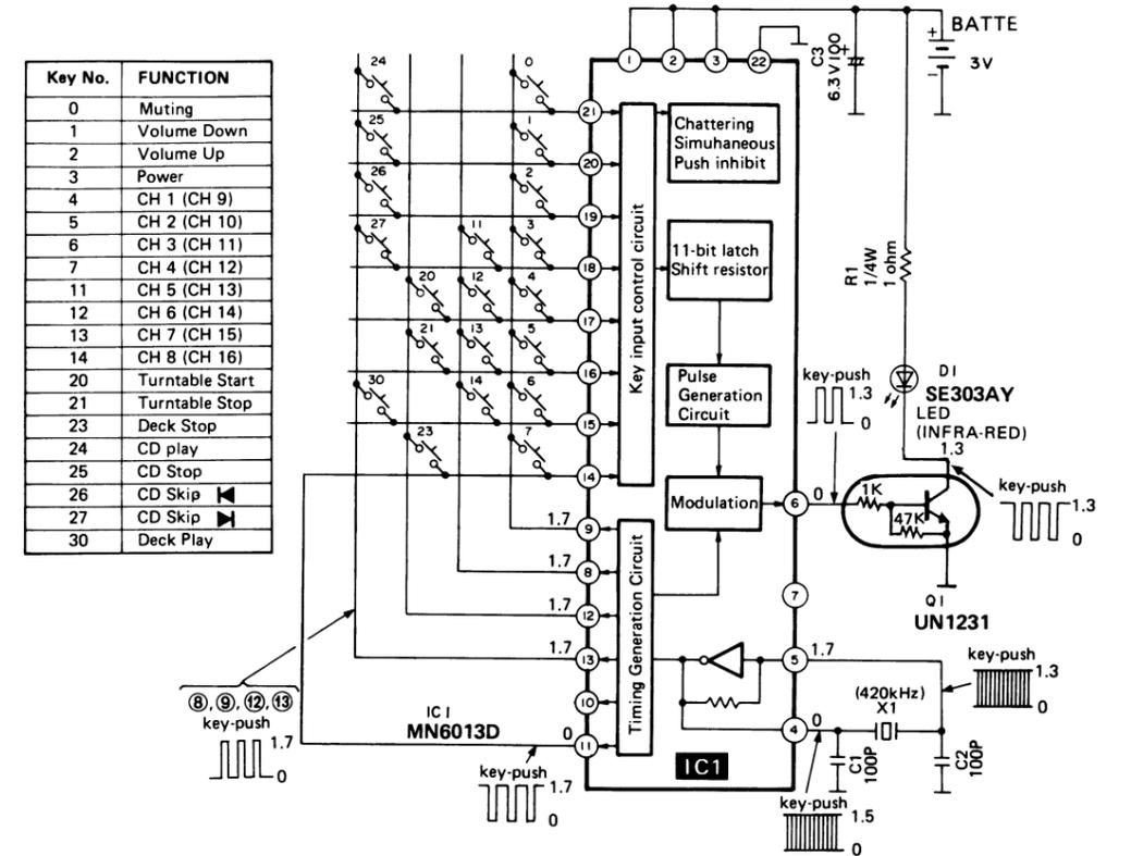
■ KEY NUMBER DESCRIPTION AND DATA CODE OF REMOTE CONTROL TRANSMITTER (Example. key No. 1)
