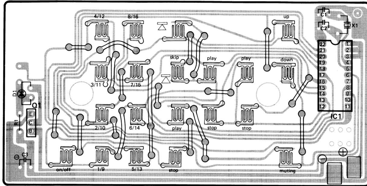
● Terminal guide of transistors, diodes and IC's
