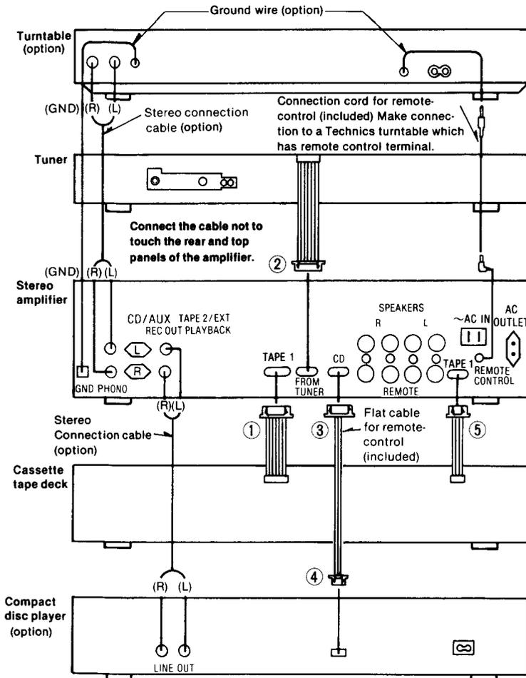
※ Flat cables for remote-control should be connected correctly. If connections are wrong, the units do not function correctly.
