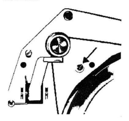
If the rubber belt rides up on the motor pulley rotate the azimuth screw counterclockwise.
