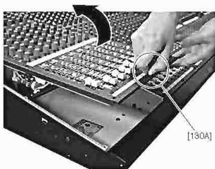
[130]: BIND HEAD SCREW-B (小ネジ+B | N D) 4.0X16 MFZN2B3 (WE968600)
