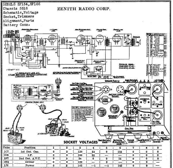
All voltages measured with a 1000 ohm per volt D.C. meter and using the Zenith 6 V Economy Pack—Antenna and ground disconnected.
